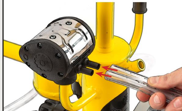
Carefully place the vacuum gauge into its designated slot on the machine, making sure not to damage it.
