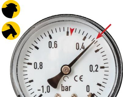
In both cases, make sure the vacuum level does not exceed -0.5 bar! If the vacuum level is incorrect, you can adjust it using the vacuum regulator on the machine.
