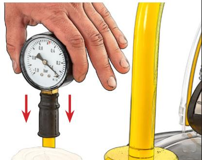
Connect the bucket and the machine. On the bucket lid, attach the tube to the inlet with the milk stopper.
