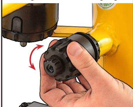
After completing the adjustment, tighten the locking nut firmly without letting the regulator body shift.
