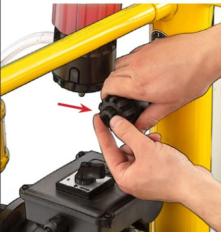
Adjust the regulator until the optimal vacuum level is reached. During the adjustment, occasionally release the regulator, as touching it can cause false readings on the vacuum gauge.
